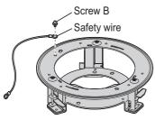
Insert the bracket into the hole in the ceiling.
